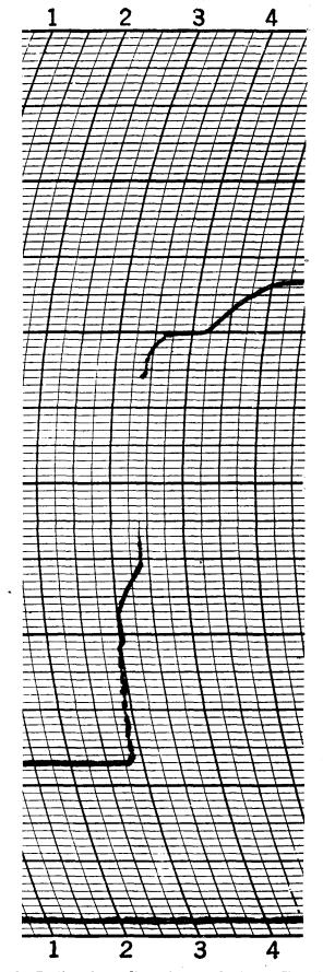
FIGURE 2.—Portion of recording rain gage chart (WB Form 1028C) showing trace of the world-record 1-minute rainfall at Unionville, Md., July 4, 1956.
